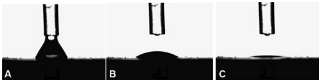
Figure 6. Penetration of water droplet into 20 kN paracetamol compacts at (a) 0 ms, (b) 950 ms, and (c) 1950 ms.
